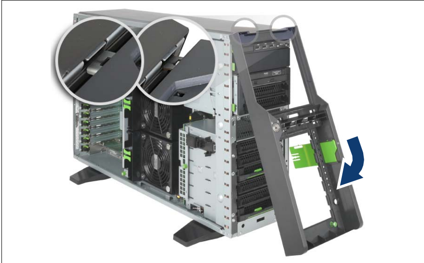
Figure 81: Attaching the front cover
